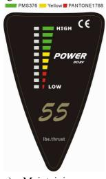
There are 10 LED on the meter, 7 upper LEDs are green and 3 lower LEDs are red, when all the green LEDs are turned off, that means the input voltage is lower than 10.25V, you must turn off the motor and disconnect the motor from the battery, otherwise it may cause forever damage to the battery.
